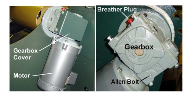
Due to the mounting configuration, the window on the gearbox cannot be used to monitor the amount of oil, however you must ensure that the gearbox is <u>never less then half filled</u> with oil at all times! Use 75W-90 synthetic gear oil, the amount required depends on the type of gearbox
